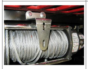
Fit the control box bracket to the winch bumper rear deck edge using the M8 bolts, washer and nuts provided.
